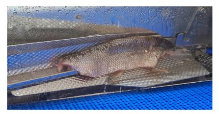
Figure 38. Curio filleting machine trial with Lake whitefish sample.
