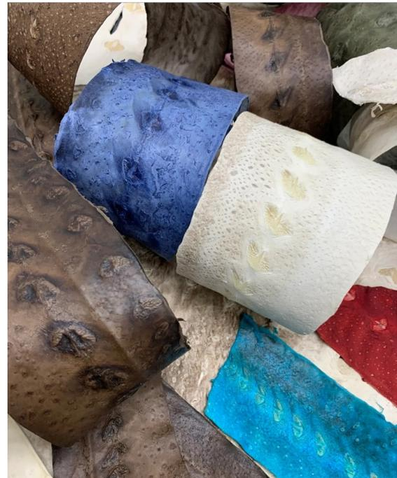
**Image 4.** Assortment of sturgeon fish leather from an industrial fish leather plant. Source: <https://theaquaborne.com/sturgeon>
